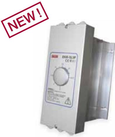
EKR15.1P is a proportional controller for multistep(up to 5 steps) electric heaters with automatic voltage adaptation. EKR15.1P controls the whole load On-Off. The ratio between On-time and Off-time is varied 0-100% to suit the prevailing heat demand.
